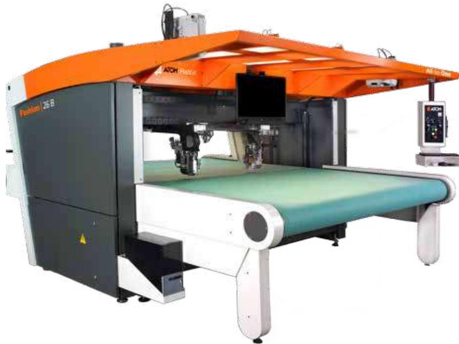
FlashCut Fashion All-in-One models combine processes of acquisition, automatic nesting and cutting in a single machine. Operating in continuous workflow, they both reduce cycle time and allow a single operator to execute all the production steps. Two independent cutting heads ensure the highest productivity in processing both half-hides and full-hides. Made for footwear, leather goods, furniture and automotive upholstery industries.
