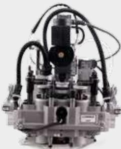
To satisfy any cutting need, the Fashion tables can cut with 5- or 7-tool heads, which can be equipped with a wide range of cutting chucks, marking pen and 3 or 5 punching tools, adjustable and rotating, with high punching frequency. The powerful Venturi system can be fitted for cutting scraps suction.
